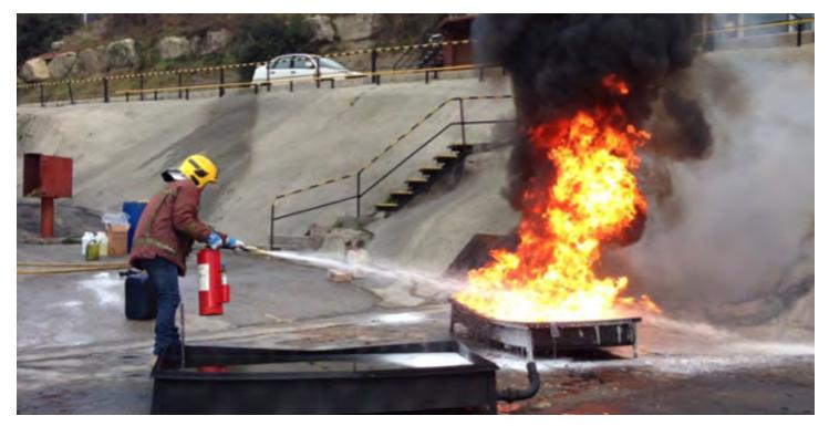
NeoSan Labs® CBRNE fuel fire test using conventional compressed air extinguisher.
